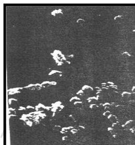
Electron Photomicrographs showing scale with antiscalant
